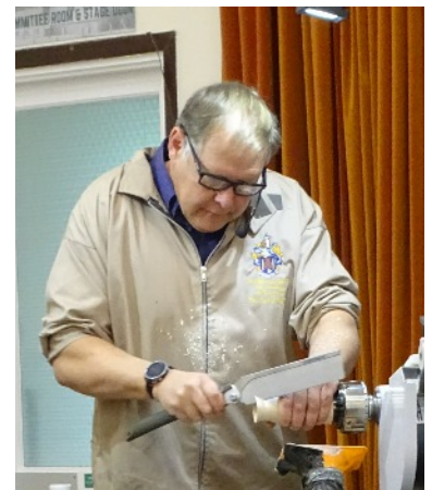
Simon sawing at an angle across the end of the top.
