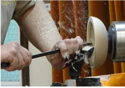
Undercutting beneath the shoulder.
