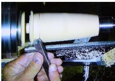
Shaping the barrel with the skew.
